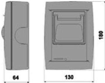
OBTPRB - Abmessungen in mm
